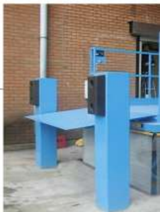
Supermarket loading bay lift
