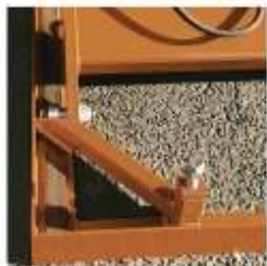
Maintenance prop in place
